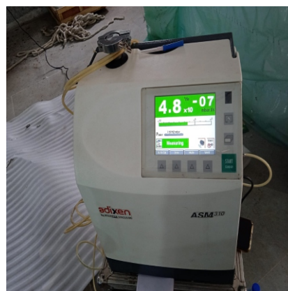
FUGITIVE EMISSION TEST
